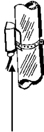
Strap sensor to pipe, firmly pressing the sensing element onto the pipe surface
